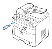
Once you have installed the USB flash drive, you can immediately print files stored on it.
