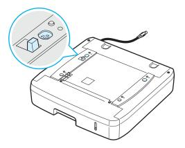
4 Place the machine over the tray, aligning the feet on the machine with the positioners on the tray.
