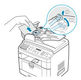
4 Align the left end of the ADF roller with the slot and push the right end of the ADF roller into the right slot (1). Rotate the bushing on the right end of the roller toward the document input tray (2).
