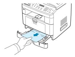
If there is any resistance and the paper does not move when you pull, or if you cannot see the paper in this area, check the fuser area around the toner cartridge. See page 9.7.
