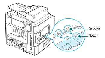
6 Push the DIMM straight into the DIMM slot until it snaps into place. Make sure the latches fit over the notches located on either side of the DIMM.
