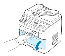
2 Lightly pushing the used cartridge down, pull it out.
