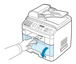
2 Pull the toner cartridge out and gently roll the cartridge 5 or 6 times to distribute the toner evenly inside the cartridge.
