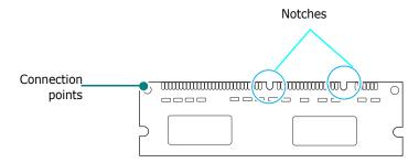
5 Holding the memory DIMM by the edges, align the notches on the memory DIMM with the grooves at the top of the memory DIMM slot.
