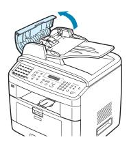
3 Rotate the bushing on the right end of the ADF roller toward the ADF  $(\widehat{1})$  and remove the roller from the slot  $(\widehat{2})$ . Pull the document gently to the left and out of the ADF.
